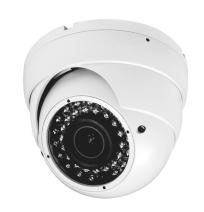
The 0E-VDIR700VW is a 700 TVL 960H Vandal Dome camera constructed with a 2.8-12mm lens and push fit structure for simple adjustment and ease of installation. Super Flux IR LEDs provide 25M IR distance and True/Day Night with ICR allows for clear night images.
